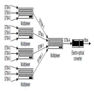
Fig 2.2.1 SDH multiplexing transmission.
