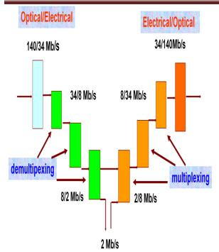
Fig.2.1.1 Optical to electrical multiplexing in UMTS network.
