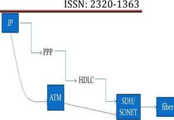
Fig .2.4.1 IP to SONET/SDH interfacing.
